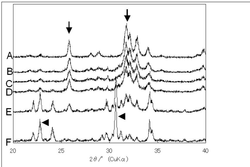
**Fig.5** X-ray diffraction of CPC powder mixed with PRP. **A**: Control (HA). **B**: On 28 days after mixing the CPC powder with PRP. **C**: On 14 days after mixing the CPC powder with PRP. **D**: On 7 days after mixing the CPC powder with PRP. **E**: On 3 days after mixing the CPC powder with PRP. **F**: CPC powder only. (arrows; HA peak, arrowheads;  $\alpha$ -TCP peak)
